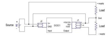
Connections for creating bi-polar supplies If isolation is not desired, connect source (-) to ouput Gnd
